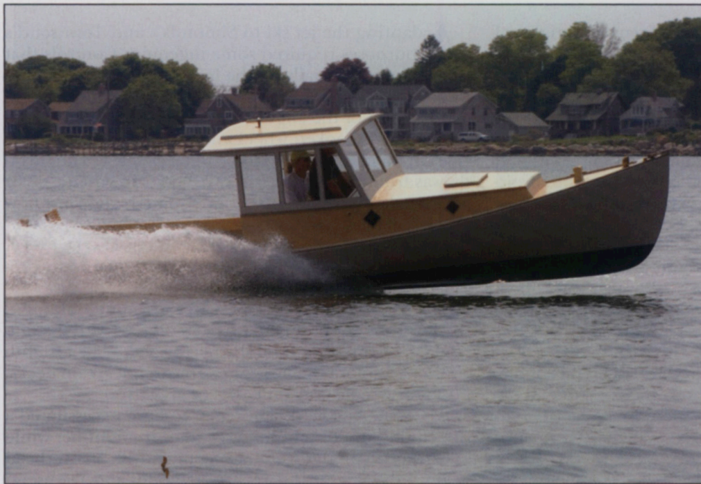
NIKI at speed. She weighs just over 2,000 lbs with full fuel and water tanks, and burns 3-4 gallons per hour at 18-20 knots.
